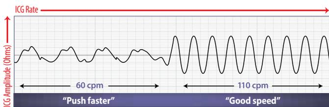
Figure 2. Rescuer's CPR compression rate is too slow, as determined by the low number of deflections detected by the ICG waveform. The SAM 450P will issue the audible prompt "Push faster" until the correct compression rate is achieved.
