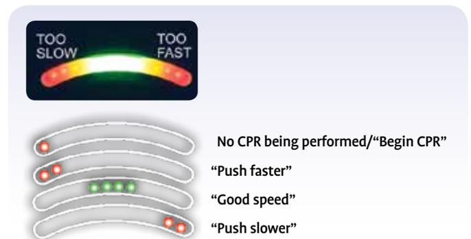
Figure 5. Visual indicators and audible feedback tell the rescuer if the rate of CPR is in line with the AHA/ERC guidelines.
