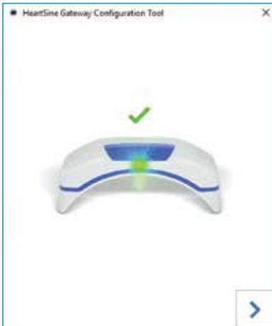
17. HeartSine Gateway will attempt to connect to the Wi-Fi network. If the connection is successful, the HeartSine Gateway status indicator will be solid green before turning off. If the connection is not successful, the indicator will begin flashing blue. In this case, it is likely the information you entered for the network was not correct and must be re-entered. Confirm that the data you have is correct and repeat each of these steps.
