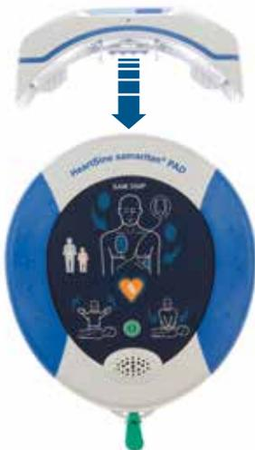
3. Slide HeartSine Gateway onto the top of the AED allowing the four pins to connect with the contacts on the data port of the AED. When HeartSine Gateway is fully connected, an audible click should be heard as the locking clips snap into place.
