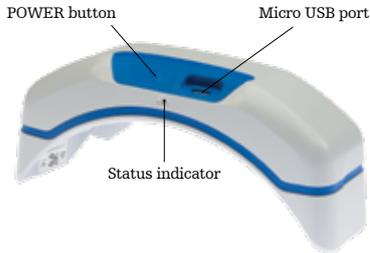
**POWER button:** Press this button to turn on HeartSine Gateway or press and hold the button for six seconds to place HeartSine Gateway into set-up mode.
