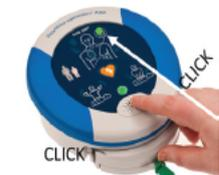
Push Pad-Pak™ into the opening and listen for the “click” sound to ensure it is properly inserted
